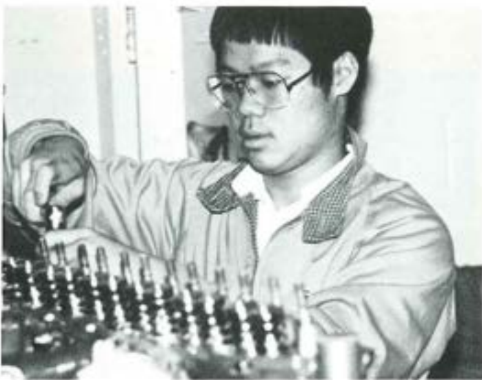
left: Springing into action Andrew Chung disassembles the valve train.
